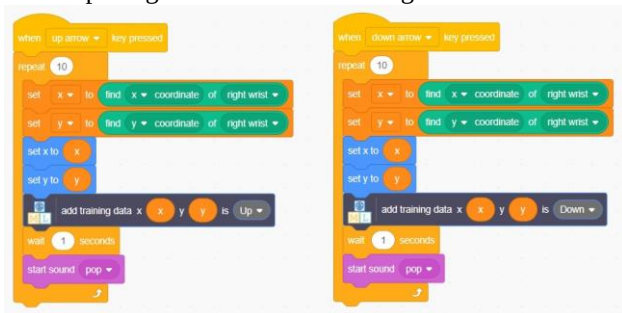
Figure 6. Scratch scripts to collect wrist up and down images
