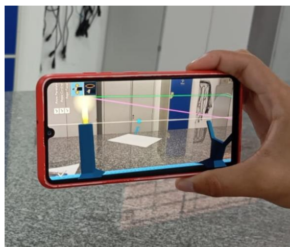
Fig. 3. Representation of the optical bench created with augmented reality.
